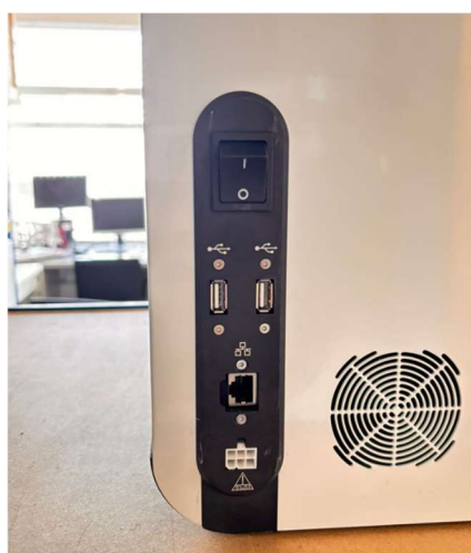
Figure 2: Connection ports. From the top: DC Switch, USB ports, Lan Cable, Power Plug
